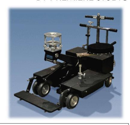
Features two steering modes, rear wheel steer and all wheel crab, with infinite crab rotation. A hydraulic accumulator system for smooth and quiet boom movement, lifting a camera with straight vertical movement.
